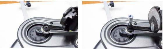
Step #4 Use an adjustable wrench on the socket end to drive the bolt into the crank thus pushing out the crank .
