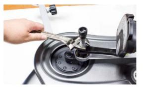
Step #3 After the hex nut is removed, insert and thread the crank puller into the now exposed socket.
