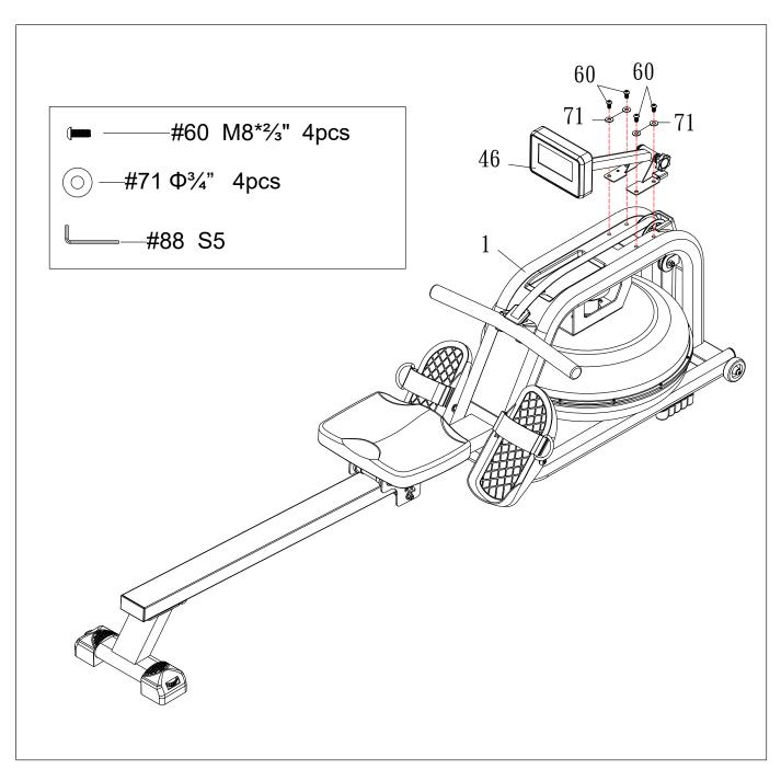
Attach the computer (#46) to Main Frame, tighten with 4 Washers (#71) and 4 Allen Bolts (#60)
