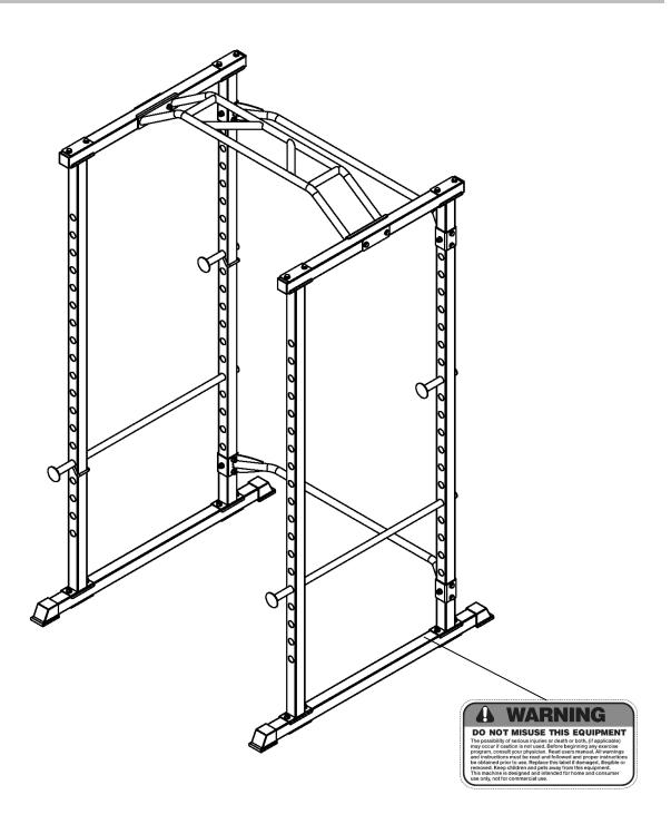
The warning labels shown here have been placed on the Base Frame. If the labels are missing or illegible, please call customer service at 1-800-999-8899 for replacements. Apply the labels in the location shown.
