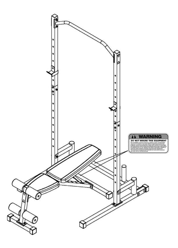
The warning labels shown here have been placed on the Cross Brace. If the labels are missing or illegible, please call customer service at 1-800-888-8899 for replacements. Apply the labels in the location shown.
