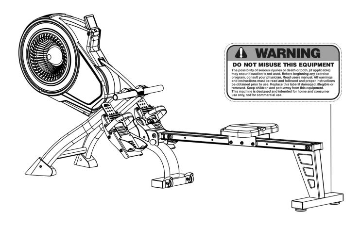
The Warning Labels shown here has been placed on the Rear Support. If the labels are missing or illegible, please call customer service at 1-800-999-8899 for replacement. Apply the labels in location shown.
