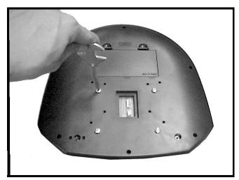
**STEP 12:**Loosen the spring washers and computer fix screws from the back of *COMPUTER (#8)*.
