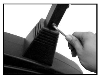
STEP 4: Insert the *COMPUTER POST (#4)* into the holder on *MAIN FRAME (#1)*. Securely tighten with three *ALLEN KEY BOLTS (D)*.
