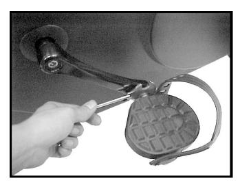
STEP 15: Connect the *RIGHT PEDAL (#13)* (marked "R") to the right crank of *MAIN FRAME (#1)*. Thread it into the crank in the clockwise direction.
