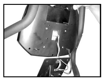
STEP 13: Attach COMPUTER (#8) onto COMPUTER POST (#4). Connect the COMPUTER WIRE (#7), SENSOR WIRE (#14) and HAND PULSE SENSOR to the back of COMPUTER (#8).
