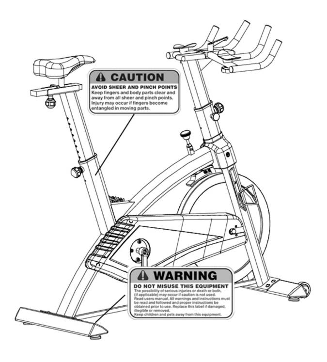
The Warning Labels and Caution Label shown here have been placed on the Rear Stabilizer and Main Frame.
