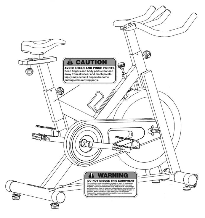
The Warning Labels and Caution Label shown here have been placed on the Rear Stabilizer and Main Frame. If the labels are missing or illegible, please call customer service at 1-800-999-8899 for replacement. Apply the labels in location shown.
