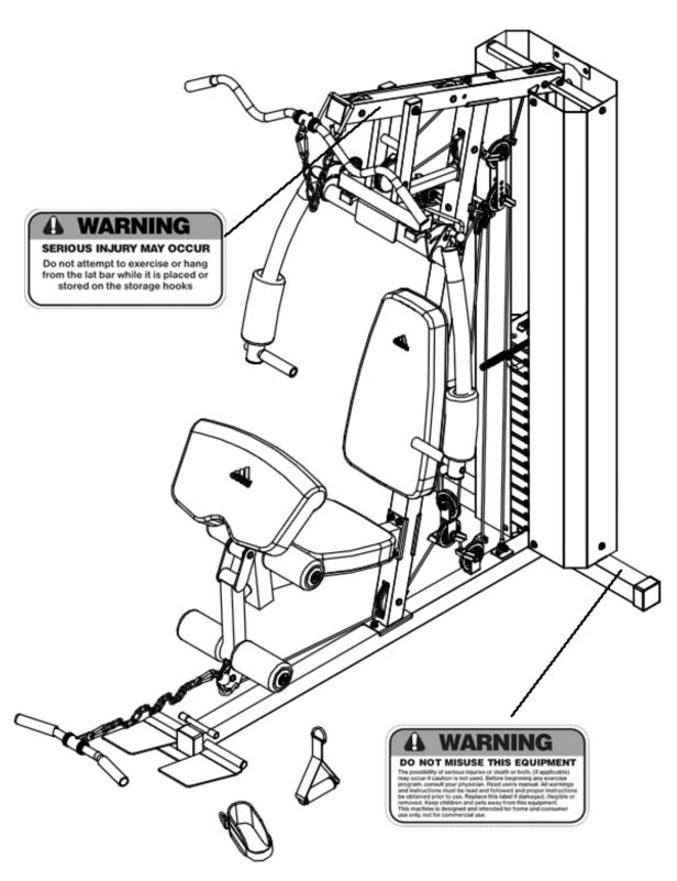
The warning labels shown here have been placed on the Rear Base and Upper Frame. If the labels are missing or illegible, please call customer service at 1-800-888-8899 for replacements. Apply the labels in the location shown.
