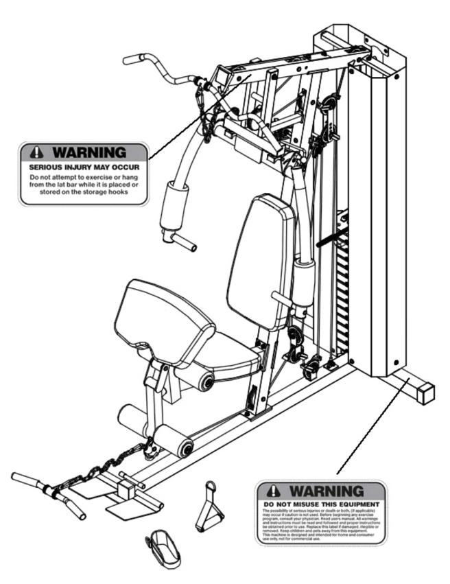
The warning labels shown here have been placed on the Rear Base and Upper Frame. If the labels are missing or illegible, please call customer service at 1-800-999-8899 for replacements. Apply the labels in the location shown.
