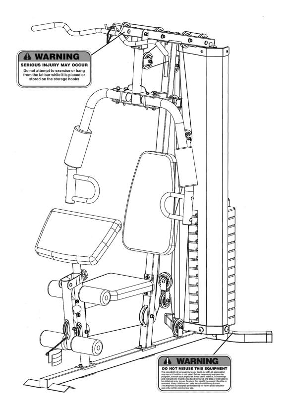
The warning labels shown here have been placed on the Rear Stabilizer and Upper Frame. If the labels are missing or illegible, please call customer service at 1-800-888-8899 for replacements. Apply the labels in the location shown.
