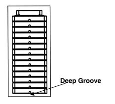
Slide weight plates onto Guide Rod from top to bottom.
