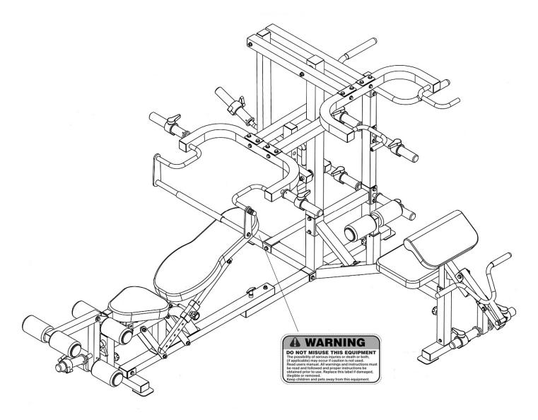
The warning labels shown here have been placed on the Base Frame. If the labels are missing or illegible, please call customer service at 1-800-888-8899 for replacements. Apply the labels in the location shown.
