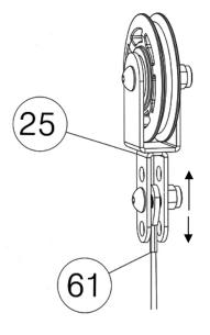
Adjust the tension of the Cable System by installingthe head of Bench Press Cable (#61) to the hole on the Single Floating Pulley Bracket (#25).
