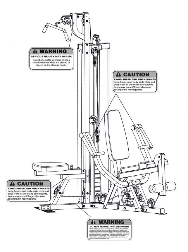
The warning labels shown here have been placed on the Base and Vertical Frame. If the labels are missing or illegible, please call customer service at 1-800-888-8899 for replacements. Apply the labels in the location shown.
