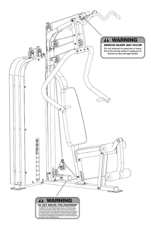
The warning labels shown here have been placed on Base Frame and Upper Frame. If the labels are missing or illegible, please call customer service at 1-866-677-4771 for replacements. Apply the labels in the location shown.
