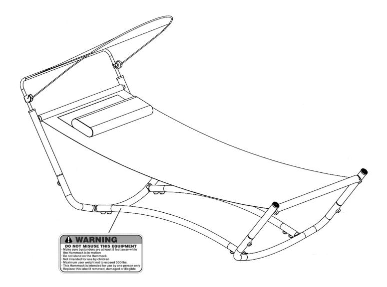
The Warning Label shown here has been placed on the Stabilizer Frame. If the label is missing or illegible, please call customer service at 1-800-999-8899 for replacement. Apply the label in location shown.
