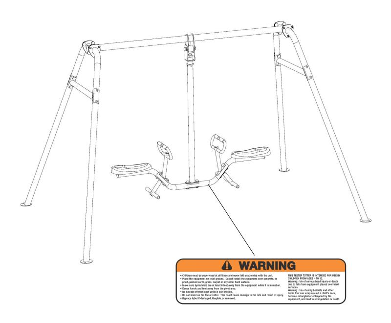
The warning labels shown here have been placed on the Base Frame. If the labels are missing or illegible, please call customer service at 1-800-999-8899 for replacements. Apply the labels in the location shown.
