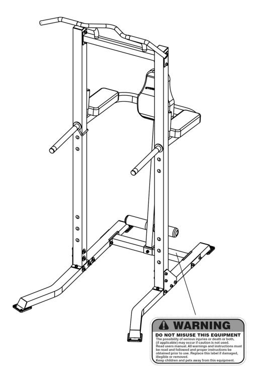
The warning labels shown here have been placed on the Cross Brace. If the labels are missing or illegible, please call customer service at 1-800-999-8899 for replacements. Apply the labels in the location shown.
