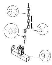
Adjust the tension of the Cable System by adjusting the length of Short Chain (#63) which is connected by C-clip (#61) to Sliding Weight Post Cable (#102).
