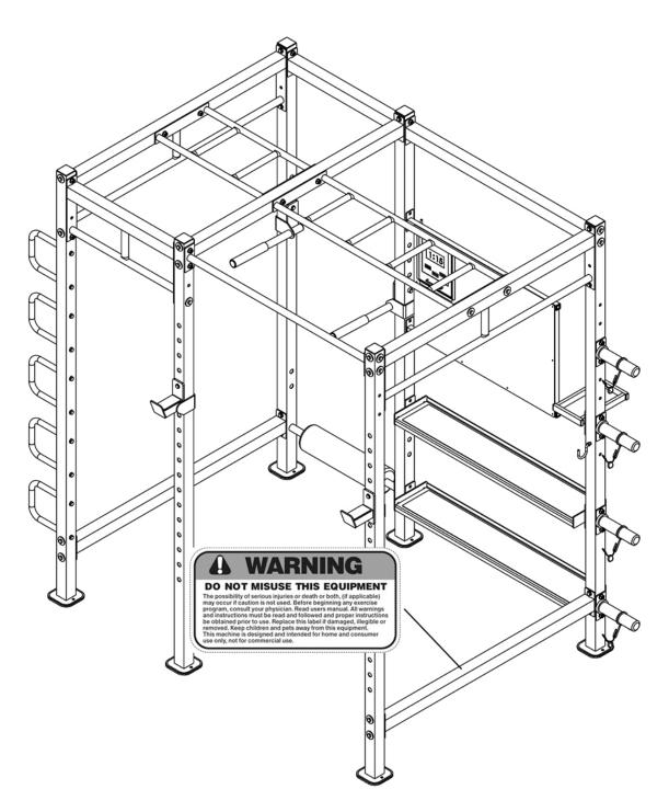
The warning labels shown here have been placed on the Lower Side Cross Brace. If the labels are missing or illegible, please call customer service at 1-800-888-8899 for replacements. Apply the labels in the location shown.
