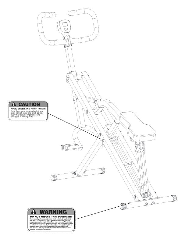
The warning labels shown here have been placed on the Base Frame. If the labels are missing or illegible, please call customer service at 1-800-999-8899 for replacements. Apply the labels in the location shown.
