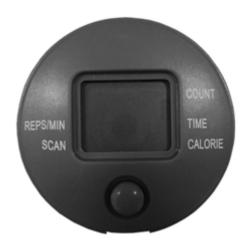
Press "SCAN" key to scan Reps/Min, Count, Time, and Calories. The display mode will change every four seconds automatically.
