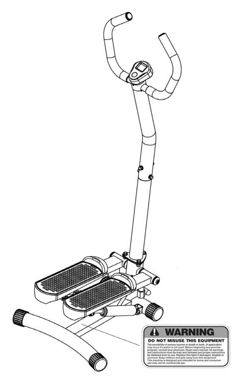
The Warning Label shown here has been placed on the Base Frame. If the label is missing or illegible, please call customer service at 1-800-999-8899 for replacement. Apply the label in location shown.
