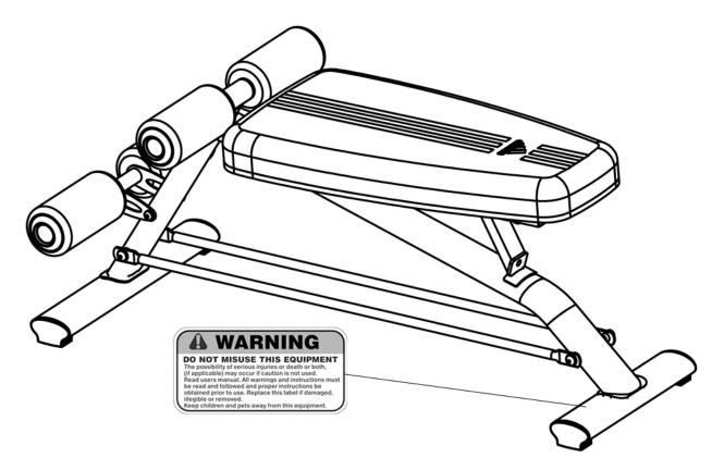
The warning labels shown here have been placed on the Base. If the labels are missing or illegible, please call customer service at 1-800-888-8899 for replacements. Apply the labels in the location shown.
