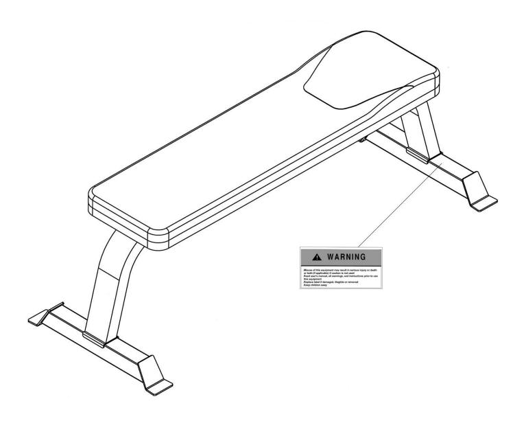
The Warning Label shown here has been placed on the Stabilizer Base. If the label is missing or illegible, please call customer service at 1-800-999-8899 for replacement. Apply the label in location shown.
