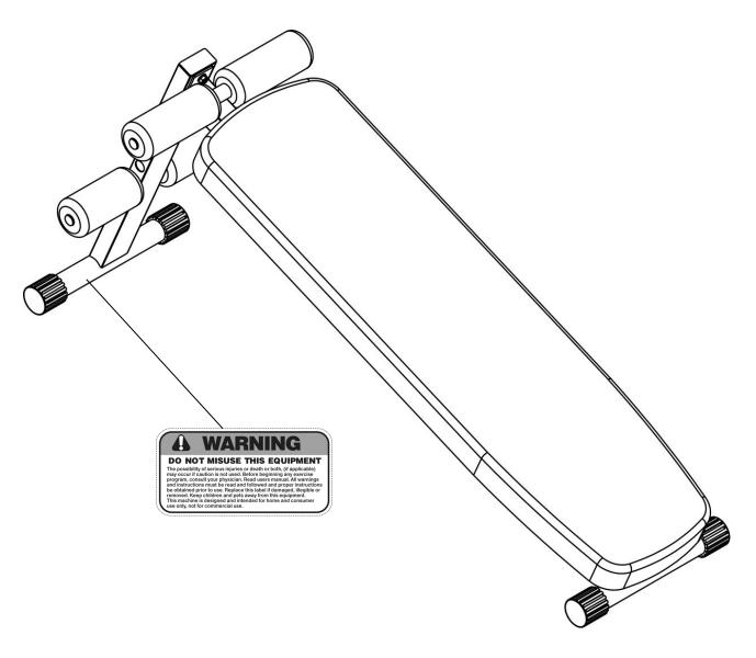
The Warning Label shown here has been placed on the Front Stabilizer. If the label is missing or illegible, please call customer service at 1-800-999-8899 for replacement. Apply the label in location shown.
