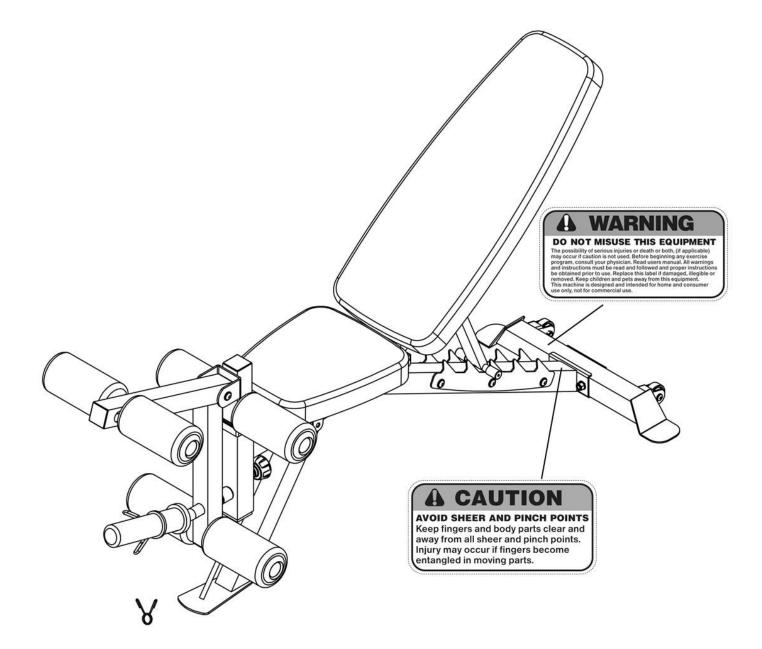
The warning labels shown here have been placed on the Rear Base. If the labels are missing or illegible, please call customer service at 1-800-999-8899 for replacements. Apply the labels in the location shown.
