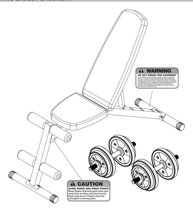
The warning labels shown here have been placed on the Rear Stabilizer and Front Post. If the labels are missing or illegible, please call customer service at 1-800-888-8899 for replacements. Apply the labels in the location shown.
