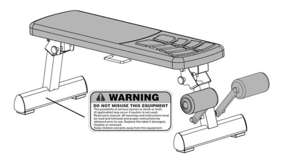
The warning labels shown here have been placed on the Rear Support. If the labels are missing or illegible, please call customer service at 1-800-888-8899 for replacements. Apply the labels in the location shown.
