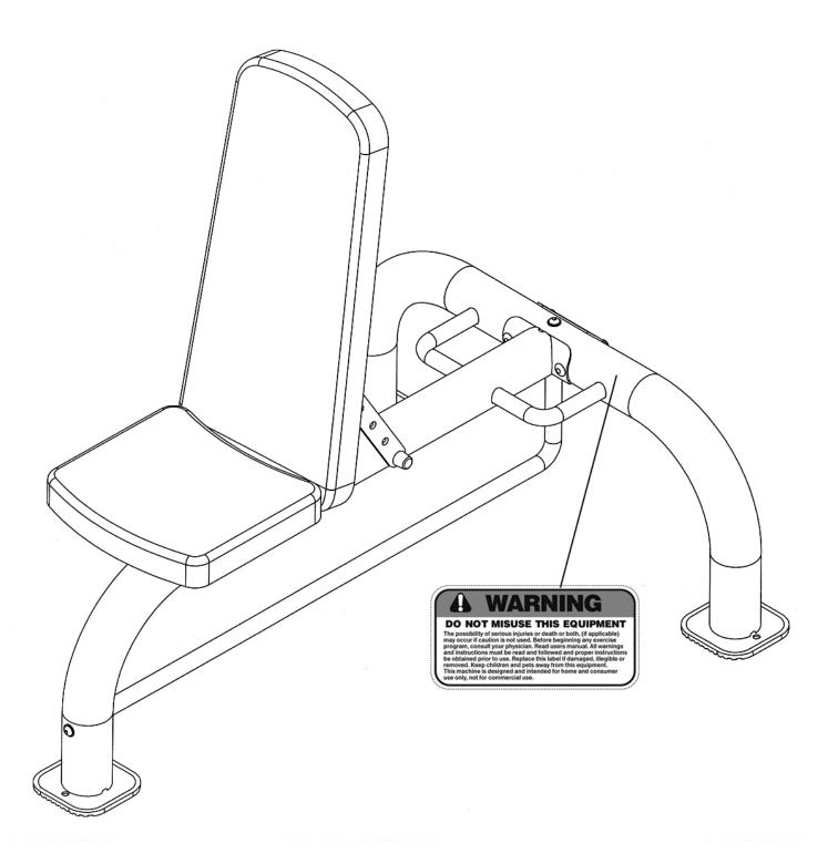
The warning labels shown here have been placed on the Rear Support. If the labels are missing or illegible, please call customer service at 1-800-888-8899 for replacements. Apply the labels in the location shown.
