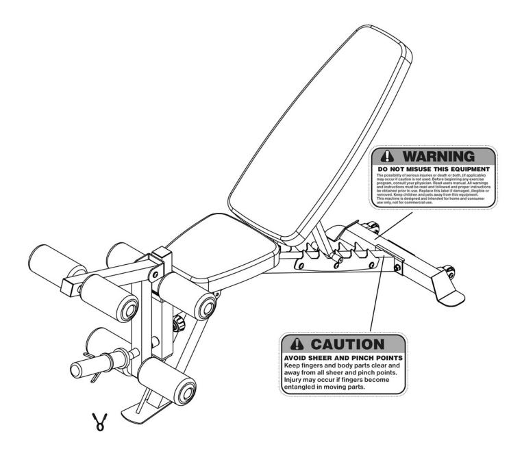
The warning labels shown here have been placed on the Rear Base. If the labels are missing or illegible, please call customer service at 1-800-888-8899 for replacements. Apply the labels in the location shown.
