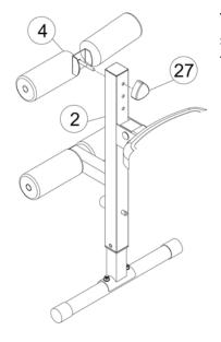
The height of Upper Leg Locking Foam Tube (#4) can be adjusted by selecting the hole on Upper Front Post (#2). Ensure the Triangular Lock is firmly lock to avoid possible injury.
