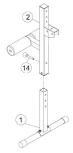
Upper Front Post (#2) height can be adjusted by selecting the hole on Lower Front Post (#1), and lock by a Lock Pin (#14). Ensure the Lock Pin is completely inserted to avoid possible injury.
