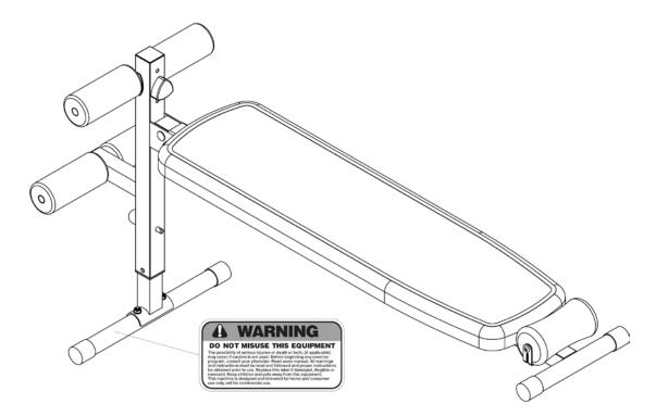
The warning labels shown here have been placed on the Front Stabilizer and Front Post. If the labels are missing or illegible, please call customer service at 1-800-888-8899 for replacements. Apply the labels in the location shown.
