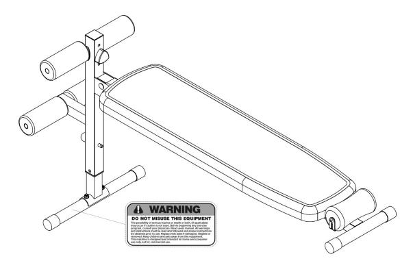
The warning labels shown here have been placed on the Front Stabilizer and Front Post. If the labels are missing or illegible, please call customer service on 1-800-999-8899 for replacements. Apply the labels in the location shown.
