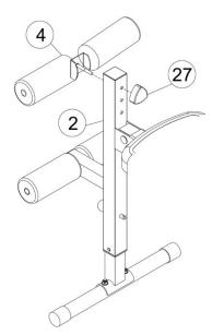
The height of Upper Leg Locking Foam Tube (#4) can be adjusted by selecting the hole on Upper Front Post (#2).
