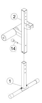
Upper Front Post (#2) height can be adjusted by selecting the hole on Lower Front Post (#1), and lock by a Lock Pin (#14).
