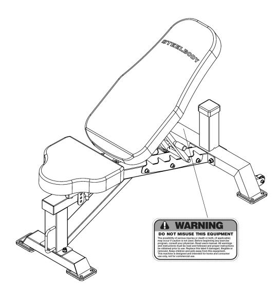
The warning labels shown here have been placed on the Rear Base. If the labels are missing or illegible, please call customer service at 1-800-999-8899 for replacements. Apply the labels in the location shown.
