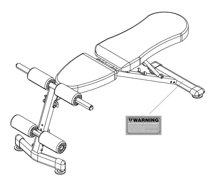
The Warning Label shown here has been placed on the Rear Base. If the label is missing or illegible, please call customer service at 1-800-999-8899 for replacement. Apply the label in the location shown.
