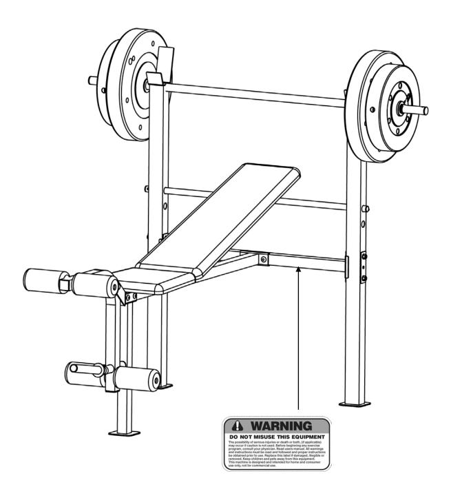
The warning labels shown here have been placed on the Cross Brace. If the labels are missing or illegible, please call customer service at 1-800-999-8899 for replacements. Apply the labels in the location shown.
