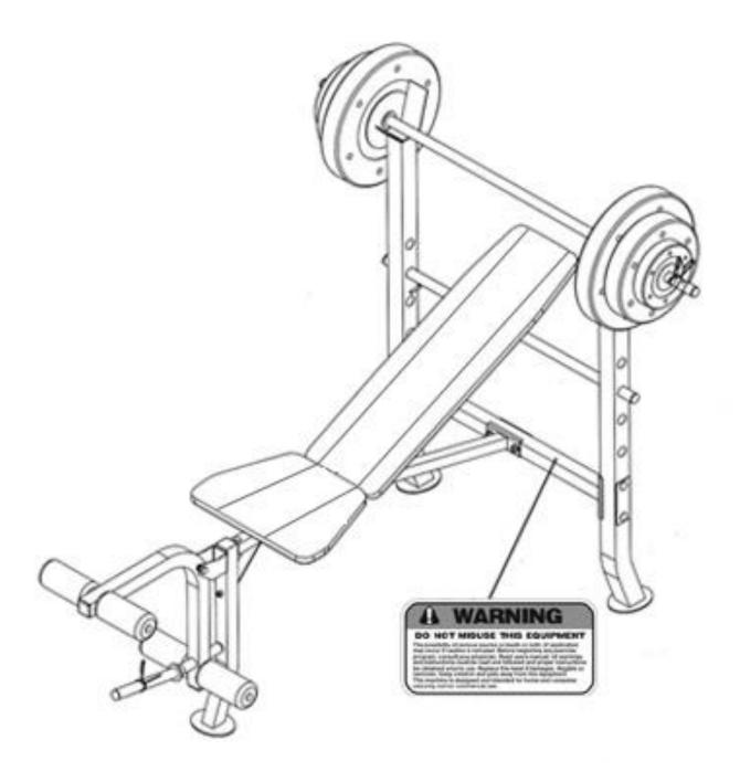
The warning labels shown here have been placed on the Cross Brace. If the labels are missing or illegible, please call customer service at 1-800-999-8899 for replacements. Apply the labels in the location shown.
