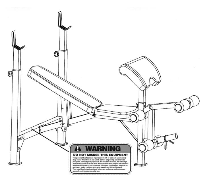
The warning labels shown here have been placed on the Cross Brace. If the labels are missing or illegible, please call customer service at 1-800-888-8899 for replacements. Apply the labels in the location shown.
