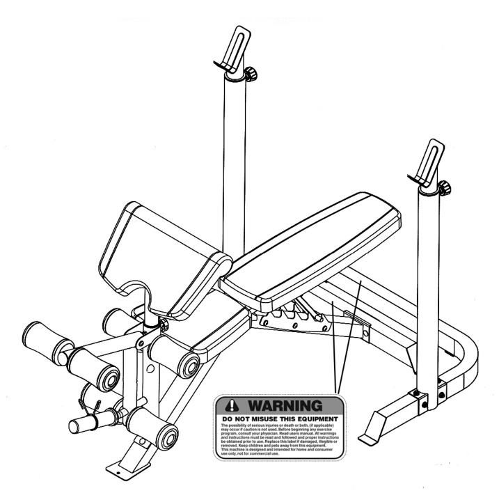
The warning labels shown here have been placed on the Cross Brace and Bench Rear Stabilizer. If the labels are missing or illegible, please call customer service at 1-800-888-8899 for replacements. Apply the labels in the location shown.
