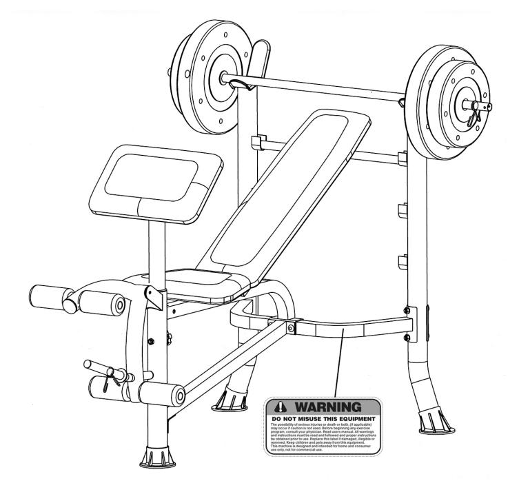
The warning labels shown here have been placed on the Cross Brace. If the labels are missing or illegible, please call customer service at 1-800-888-8899 for replacements. Apply the labels in the location shown.
