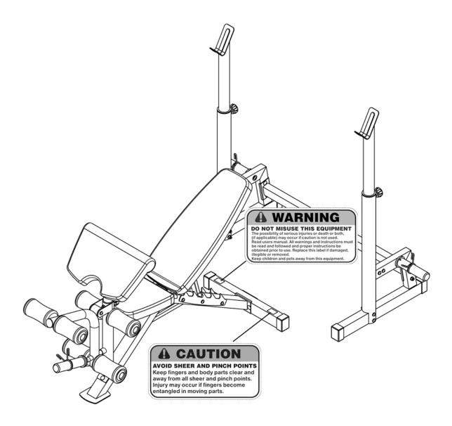
The warning labels shown here have been placed on the Rear Base. If the labels are missing or illegible, please call customer service at 1-800-888-8899 for replacements. Apply the labels in the location shown.
