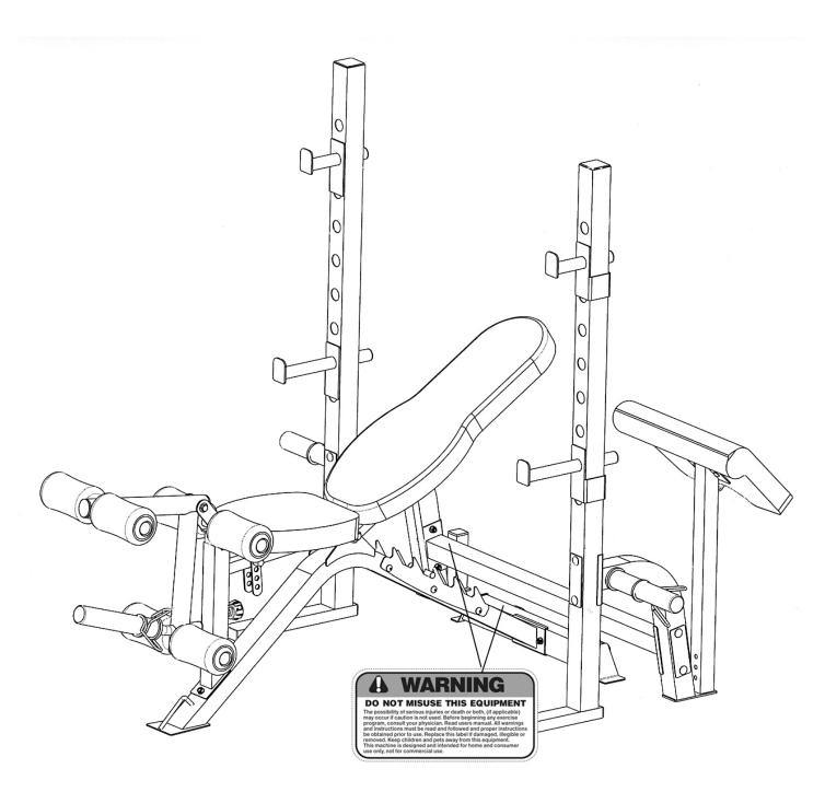
The warning labels shown here have been placed on the Cross Brace and Rear Base. If the labels are missing or illegible, please call customer service at 1-800-888-8899 for replacements. Apply the labels in the location shown.
