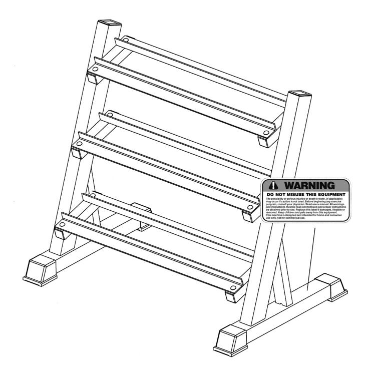
The Warning Label shown here has been placed on the base of Upright Beam. If the label is missing or illegible, please call customer service at 1-800-999-8899 for replacement. Apply the label in location shown.
