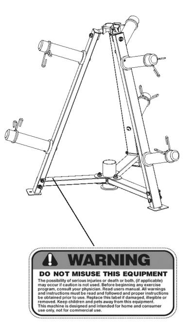
The warning labels shown here have been placed on the Cross Brace. If the labels are missing or illegible, please call customer service at 1-800-999-8899 for replacements. Apply the labels in the location shown.
