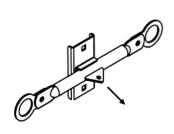
When assembling the Connecting Frame (Part#4), the triangular bracket on the Connecting Frame (Part #4) needs to point downward.
