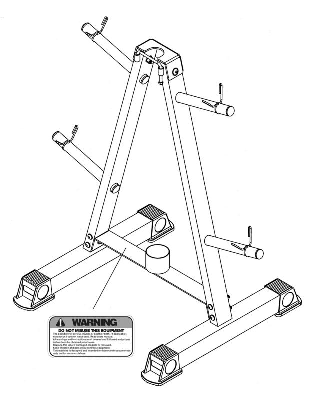
The warning labels shown here have been placed on the Cross Brace. If the labels are missing or illegible, please call customer service at 1-800-888-8899 for replacements. Apply the labels in the location shown.
