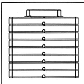
Slide weight plates onto Guide Rod from top to bottom.
