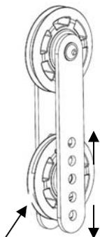
Adjust the tension of the Cable System by moving the lower Pulley position on the Double Floating Pulley Brackets.
