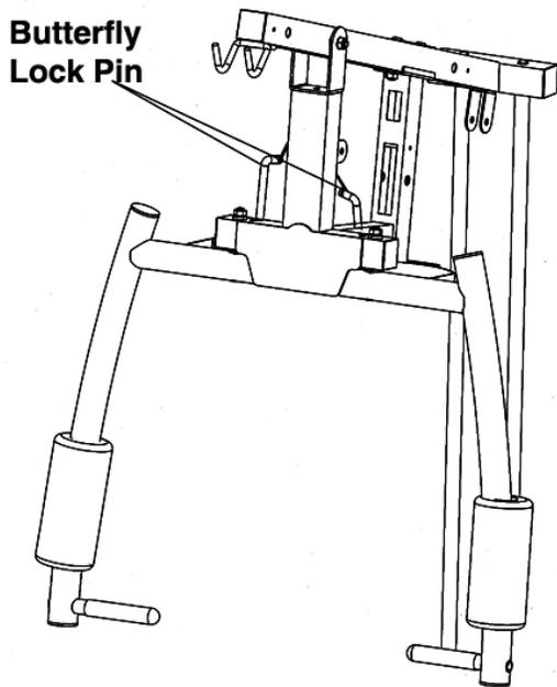
1. Insert the Butterfly Lock Pin through the holes on Front Press Base and Butterfly to lock the Butterfly in position when doing Front Press exercises.
