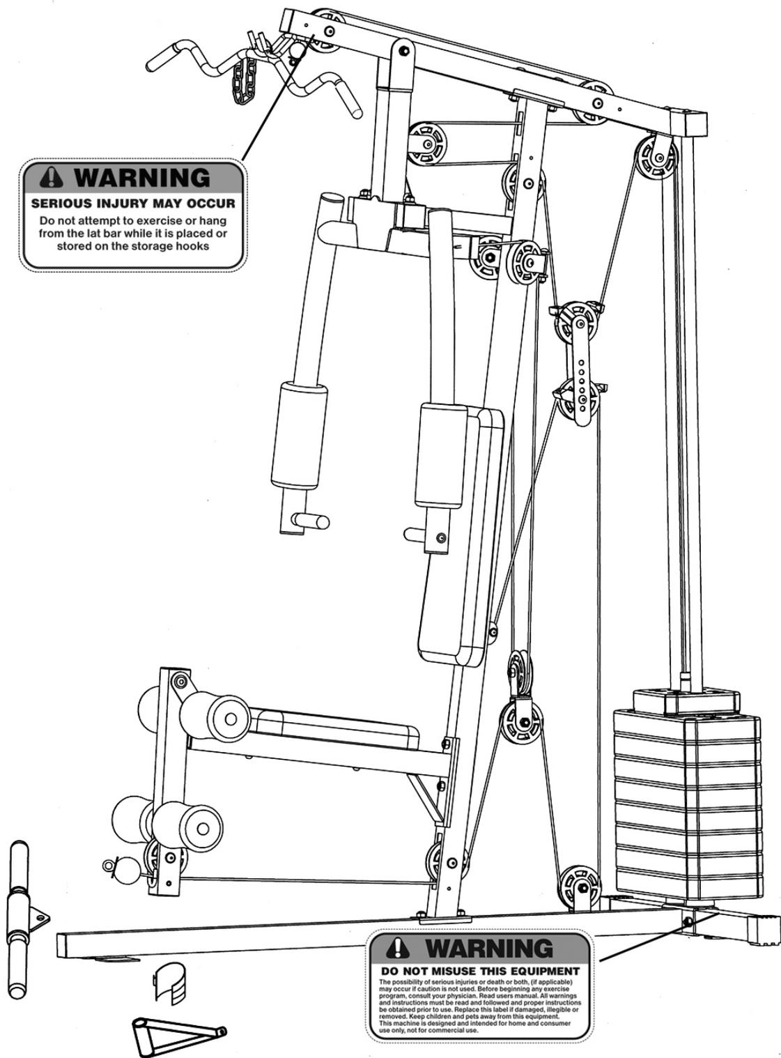
The warning labels shown here have been placed on the Rear Base and Upper Frame. If the labels are missing or illegible, please call customer service at 1-800-888-8899 for replacements. Apply the labels in the location shown.
