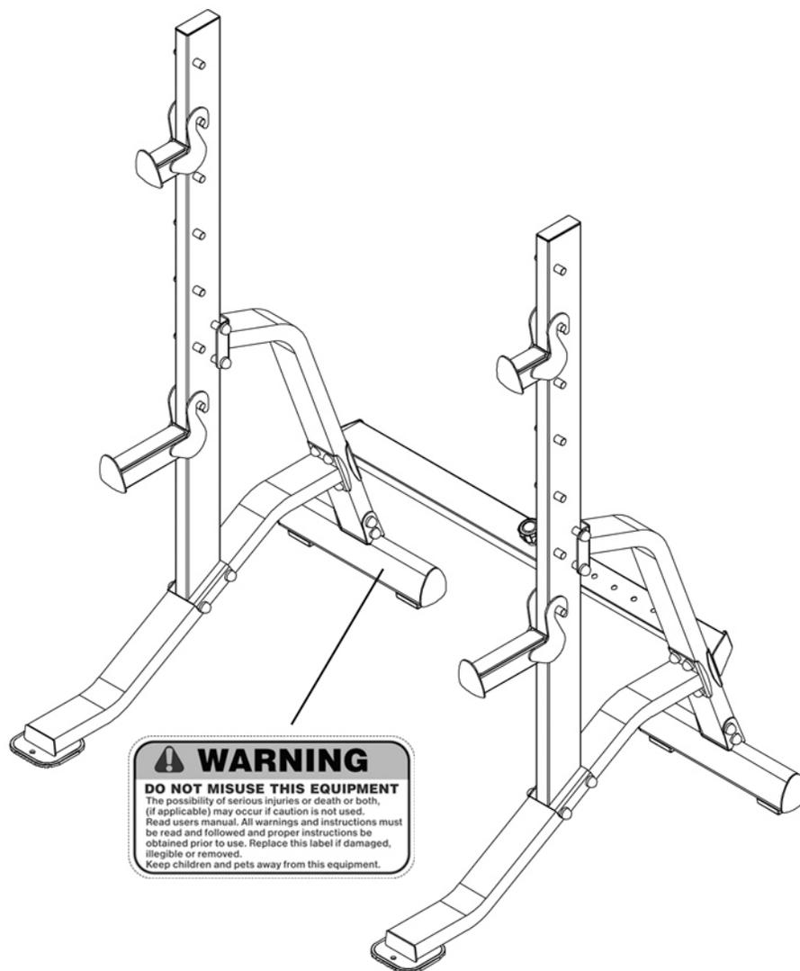
The warning labels shown here have been placed on the Rear Base. If the labels are missing or illegible, please call customer service at 1-800-888-8899 for replacements. Apply the labels in the location shown.
